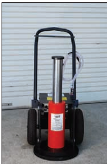
ToughLift TL100A530 fitted with non locking extension.
