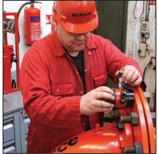
Above: Practical training in use of Hi-Force hydraulic bolt tensioning system at the Hi-Force UK office.
