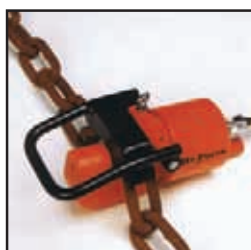
Picture 2: HCC26 cutter shown with swivel action safety guard closed.
